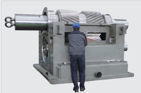
CUSTOMER : US Steel Co., Ltd. PRODUCT & SPEC : PINION STAND APPLICATION : STEEL MILL CAPACITY : 1,150,000 N.m (2,850 x 2,700 x 2,500) WEIGHT : 45,000kg
