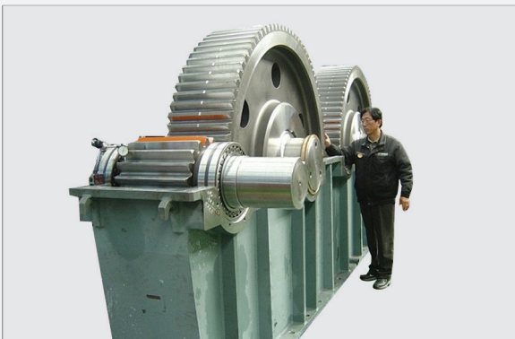
CUSTOMER : DOOSAN HEAVY INDUSTRIES Co., Ltd. PRODUCT & SPEC : MAIN HOISTING REDUCER / 700TON APPLICATION : TRANSPORTING PRODUCTS CAPACITY : 460,000 N.m (800 x 2,300 x 5,300) WEIGHT : 21,000kg
