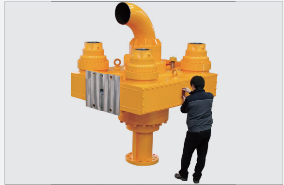
CUSTOMER : SAMBO C.M.C PRODUCT & SPEC : R.C.D GEAR BOX APPLICATION : R.C.D (Reverse Circulation Drilling Machine) CAPACITY : 800,000 N.m (2,100 x 2,300 x 2,800) WEIGHT : 14,000kg
