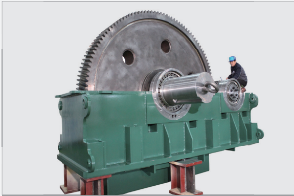
CUSTOMER : HYUNDAI HEAVYIND. Co., Ltd. PRODUCT & SPEC : REDUCER GEAR BOX APPLICATION : STEEL MILL CAPACITY : 1,150,000 N.m (4,800 x 3,000 x 3,750) WEIGHT : 53,000kg
